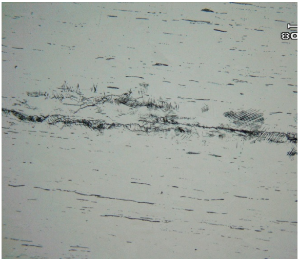
Figure 3. Cracking along non metallic inclusions
