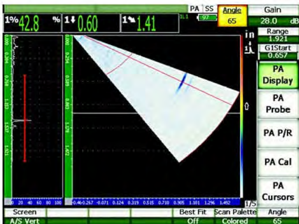
Figure 4-8 Response prior to gain normalization
