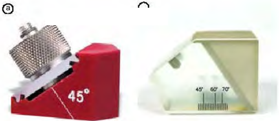
Figure 5-15 Beam index points on a conventional wedge (a) and phased array wedge (b)
