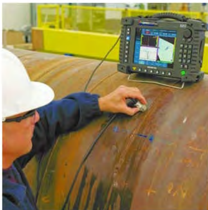
Figure 5-1 Typical phased array inspection using the OmniScan
