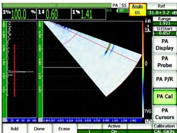
Figure 4-9 Response following gain normalization
