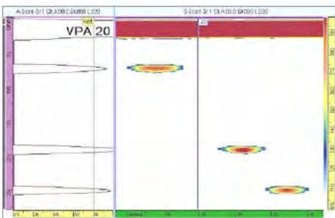
Figure 5-5 Normal beam linear scan image with all laws A-scan
