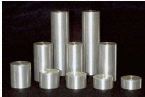
Distance/area amplitude correction blocks typically are purchased as a ten-block set, as shown above. Aluminum sets are manufactured per the requirements of ASTM E127 and steel sets per ASTM E428. Sets can also be purchased in titanium. Each block contains a single flat-bottomed, plugged hole. The hole sizes and metal path distances are as follows:
