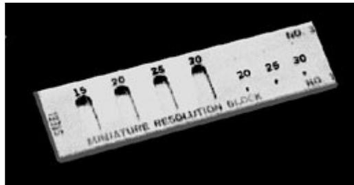
The miniature resolution block is used to evaluate the near-surface resolution and sensitivity of a normal-beam setup. It can be used to calibrate high-resolution thickness gages over the range of 0.015 inches (0.381 mm) to 0.125 inches (3.175 mm).
