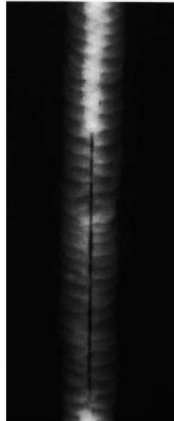
Incomplete - or Lack of Penetration (L.O.P.) A darker density band, with very straight parallel edges, in the centre of the width of the weld image.
